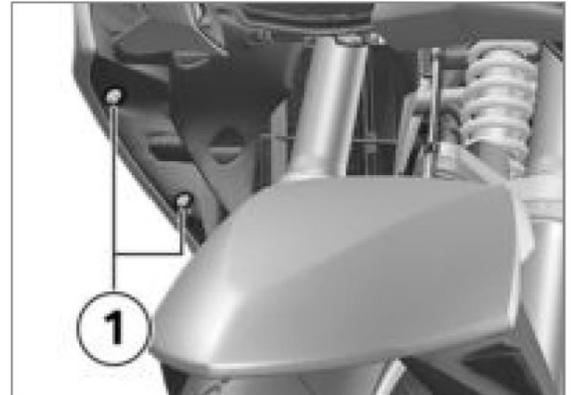
When removing and installing RH panel, note the tabs that are on the rear facing edge of the panel, which require the panel to be pulled-out at the front (rubber grommet prongs), then moved back to "unhook" the two tabs on the panel.
