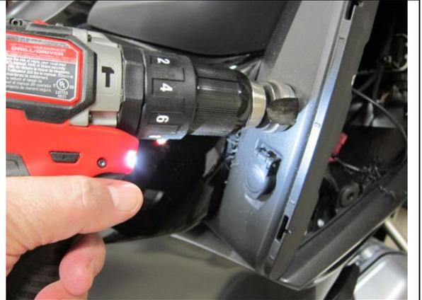
Install lighter socket through hole, install nut behind and tighten, correcting plug and weatherproof cover alignment as desired.
